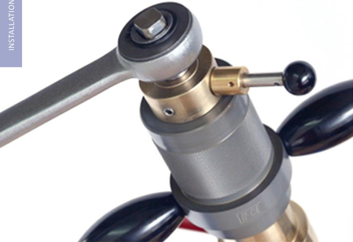
The hot tap drill is the universal tool to install your insertion flow meter in any compressed air system. In only 30 minutes you can drill a hole and install your flow meter. Using a hot tap saddle and a hot tap drill, you can create a new installation point without depressurizing your installation. The VPInstruments hot tap drill can be used for drilling through a hot tap saddle with a 1" fitting.
