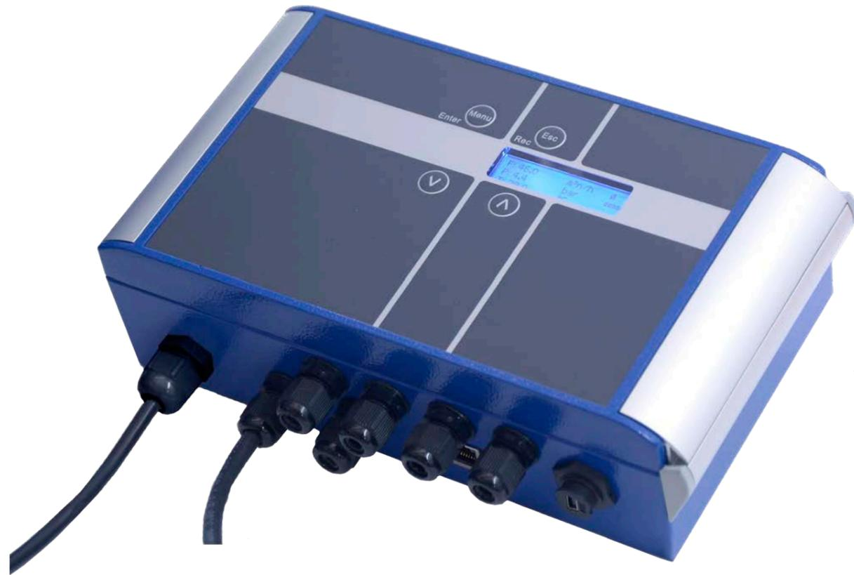
The VPFlowTerminal is a plug & play wall mount display with built-in power supply and 2 million point data logger. The VPFlowTerminal has 5 sensor inputs: 1 input for a VPFlowScope In-line, Probe or DP, and 4 generic analog inputs. It can record up to 8 channels. This makes the collection and analysis of your compressed air data easier and quicker!
